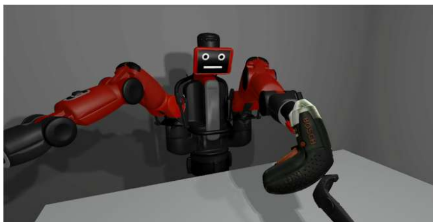
Figure 1. Top: Example VR robot models arranged according to their anthropomorphism. R0: one arm basic; (R1) an articulated arm; (R2): two arms Baxter; (R3): a humanoid robot. Bottom: an example VR-collaboration scene used by the authors, developed with Unity Game Engine (Unity Technologies, San Francisco, CA, USA). The scene shows a basic tool-passing task in which subject kinematic and physiological data can be recorded in response to manipulated scene features (e.g., cobot appearance, speed, etc.).
