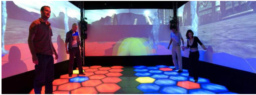
Fig. 5. XIM Multiuser Interaction Scenario: Multiple real users interacting with each other in a mixed reality Pong game, which is one of the scenarios used to evaluate PASAR's performance. Also remote users take part in the same interaction by logging in from remote machines into the virtual world and they are represented by avatars on the projection screens (adapted from [31]).
