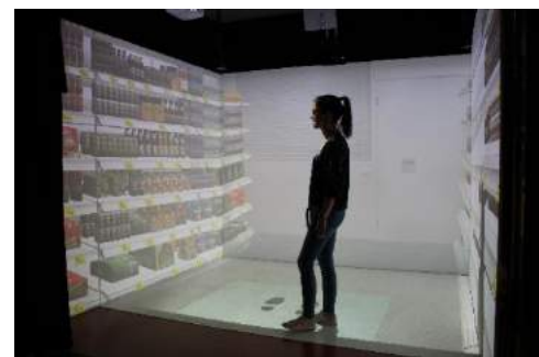
Fig. 3. Low-cost CAVE powered by the KAVE software.
