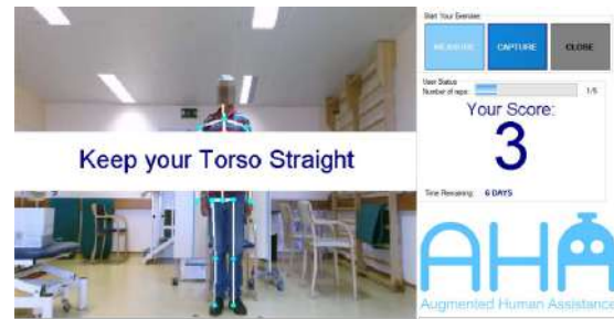
Figure 1: Computer-assisted stroke rehabilitation tool to assess the quality of patient's exercise using machine learning algorithms and a Kinect.
