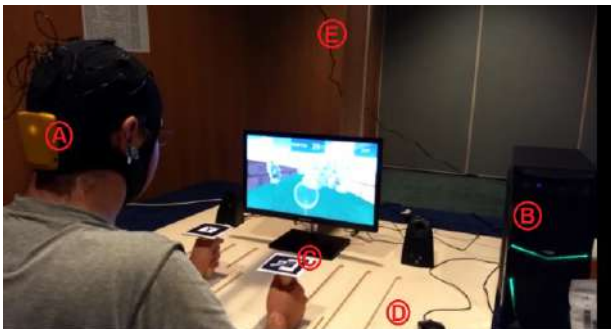
Fig. 2. Physical setup including A. EEG system; B. Computer; C. Tags for being tracked; D. Wood surface structure; E. Tracking Camera (Above structure, not visible in the image)
