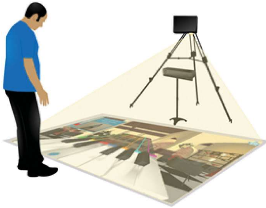
Figure 1. Experimental setup. The user interacts with a floor projection while his movements are being tracked by a Kinect sensor.
