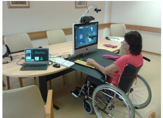
Fig. 5. Patient interacting with the VR training using AnTS. Left: the CP and AnTS running on the experimenters PC for data acquisition, logging, filtering and transmission. Right: The patient with a colored glove for tracking, interacting with TPT-VR
