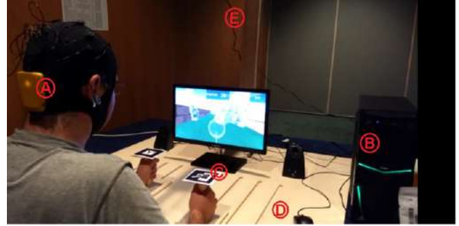
Fig. 2. Physical setup including A. EEG system; B. Computer; C. Tags for being tracked; D. Wood surface structure; E. Tracking Camera (not visible in the image)
