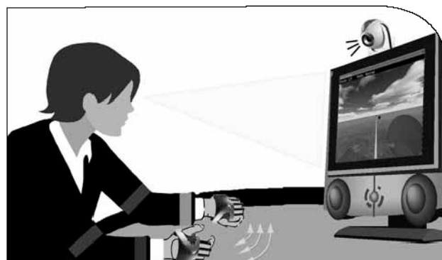
FIGURE 1. The Rehabilitation Gaming System (RGS) setup. The RGS constitutes a standard paradigm comprising all the key elements of any VR based cognitive-neurorehabilitation system. Motion capture is achieved through a video based system. The user wears color patches that are tracked by the motion capture system and that are mapped onto a virtual character through a biomechanical model. Data gloves provide finger flexion data. The screen displays a first person view of the gaming scenario in the virtual environment. The versatility of the used gaming technology (Torque, Garage Games, www.garagegames.com ) allows the rapid development of new rehabilitation scenarios.
