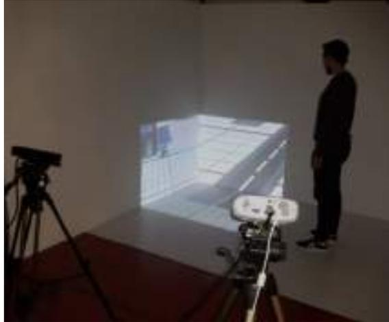
Fig. 8. Improvising a minimal CAVE with a corner projection.
