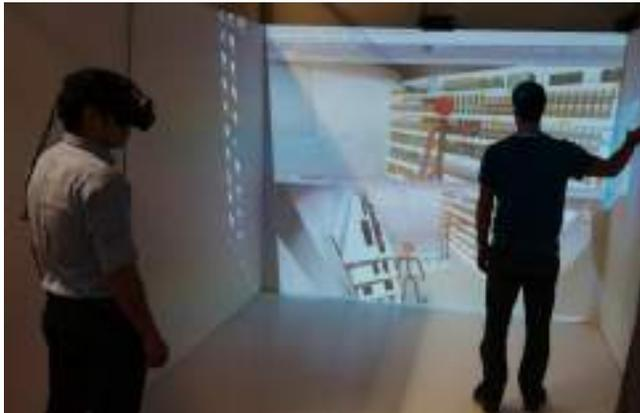
**Fig. 10. The KAVE plugin enabling an HMD wearer to see his own virtual body and others tracked by the Kinect. The HMD view and perspective view of the scene are being exceptionally projected on the front wall, top and bottom half respectively.**
