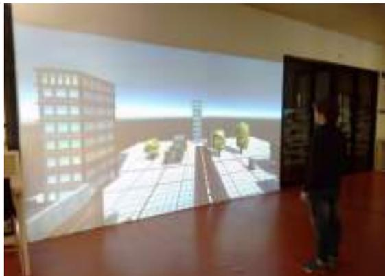
**Fig. 7. Interactive Wall, 4.84 m by 2 m of 2 projectors.**
