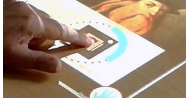
Figure 1: Circular timer and marker. A blue circular timer is activated after occluding the marker with the finger, full body or random physical objects.
