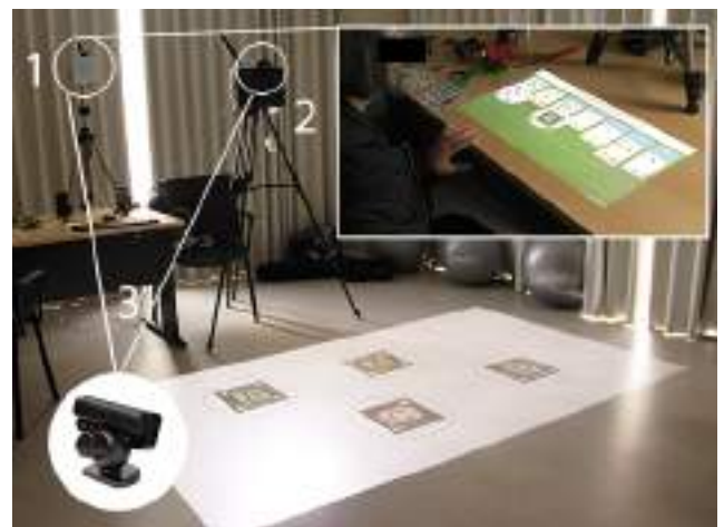
Figure 2: System configuration(s). (1) Table projection setup with a projector and a tripod. (2) Floor projection setup through a high-intensity projector and a tripod. (3) A PsEye camera which is collocated with the projectors to track and identify the projected markers A, B, C and D.
