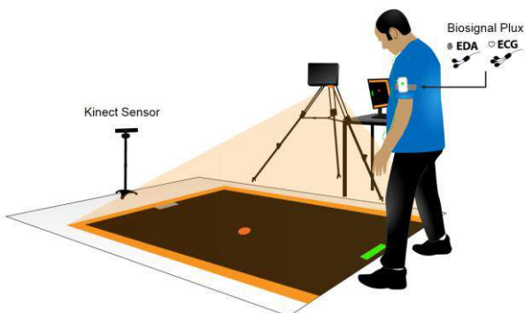
Figure 1. Diagram depicting the Exerpong setup consisting of a Kinect sensor, a projected environment and a wearable physiological kit. The user stands in front of the projection and controls a virtual paddle.
