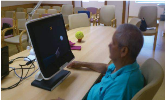
Figure 1. Experimental setup being used by a stroke patient, consisting of a monitor with an integrated eye tracker running a custom made virtual reality environment.
