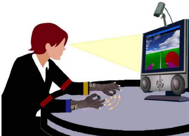
Fig. 1. The Rehabilitation Gaming System. A subject sits on a chair with his/her arms resting on a table and facing a screen. Arm movements are tracked by the camera mounted on top of the display. The tracking system determines in real-time the position of the color patches positioned on the wrists and elbows and maps these onto a biomechanical model of the upper extremities. Data gloves are used to detect finger movements. Thus, on the display two virtual arms reproduce the movements of the subject's arms.
