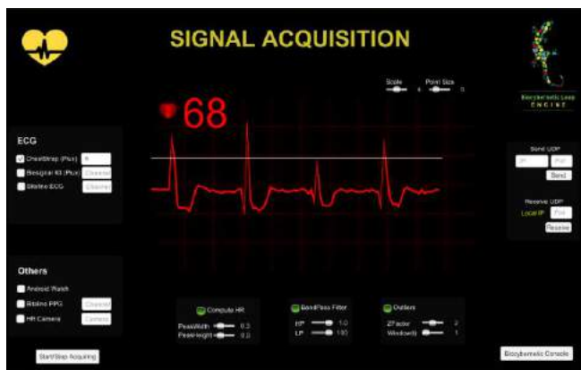
Figure 6. The Biocybernetic Loop Engine tool illustrating the acquisition panel (left) for getting HR from different sensors and the biocybernetic console (right) for the creation of physiologically-adaptive rules.
